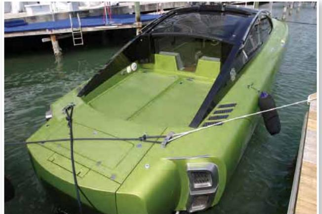
*Open and shut: The 42's cabin is completely enclosed, above. Then, in seconds, a remote-control device quickly slides open the roof and entrance panel, below.*
